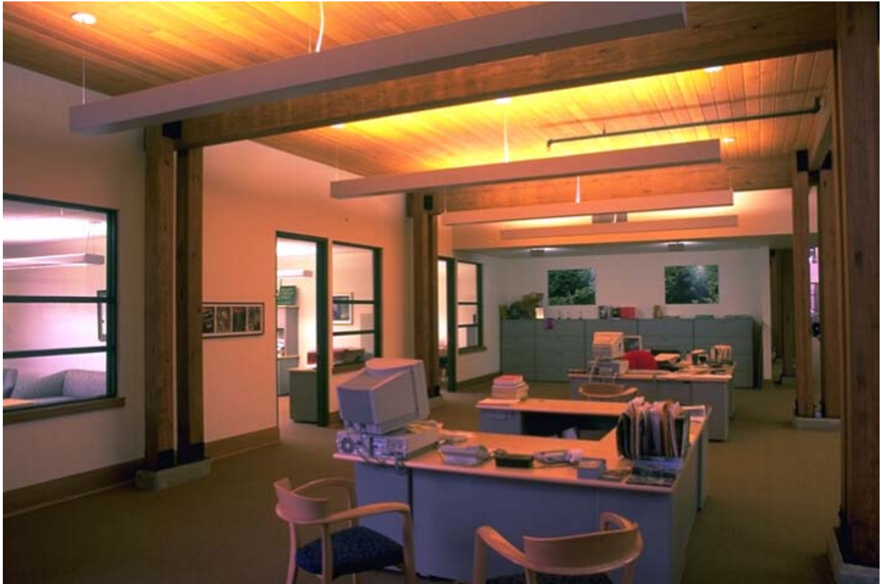
Figure 4 Minimize direct glare with indirect lighting.
